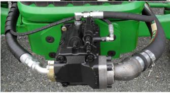
Piston Pump Hydraulics—2" Suction Hose
