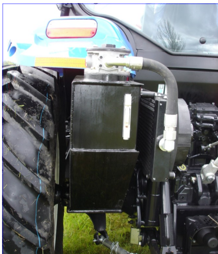
55,000 BTU Cooler w/ Fan mounted to 25 gallon tank
