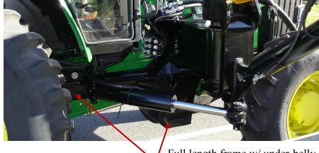
Full Frame Support Travel Rest Full length frame w/ under-belly structural support. No bolts into right side bell housing
