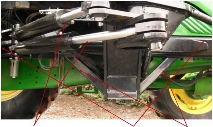
Dual Swing Cylinders 220° Swing Arc Full Frame Support Travel Rest
