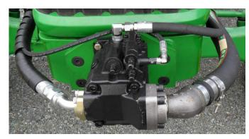
Piston Pump Hydraulics 2" Suction Hose
